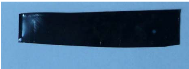
Fig. 1 Carbon–TiC composite film (TC-10w) produced by heat treatment, for 5 h at 1,600 °C, of PI/TiC composite with 10 wt% TiO 2
